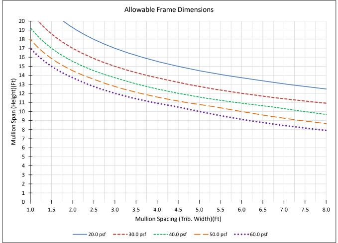
Using this chart: Plot the mullion height (span) and the intended mullion spacing. If mullion spacing is uneven, add the DLO width on each side of the mullion and divide by 2. Plotted points below a given curve are acceptable for that design pressure (PSF). Plotted points above a given curve will require a heavier mullion or reinforcing for that design pressure (PSF).
