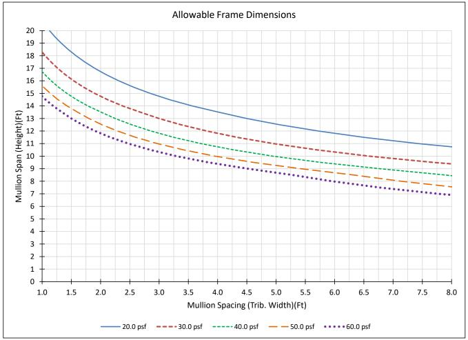
Using this chart: Plot the mullion height (span) and the intended mullion spacing. If mullion spacing is uneven, add the DLO width on each side of the mullion and divide by 2. Plotted points below a given curve are acceptable for that design pressure (PSF). Plotted points above a given curve will require a heavier mullion or reinforcing for that design pressure (PSF).
